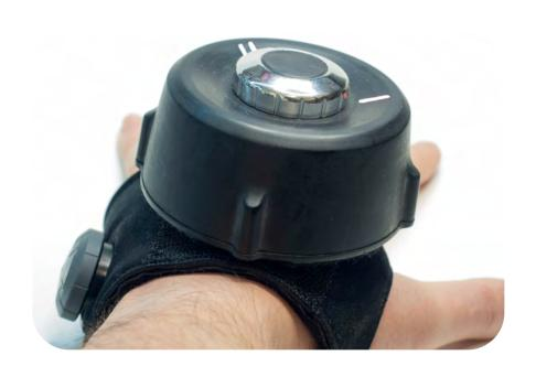
Step 5: Align the bottom center of the Stabiliser unit with the small round circle at the top of the glove. Bring the Stabiliser closer, and it will magnetically attach itself to the glove.
